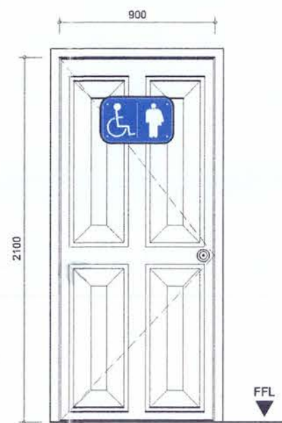
D1 PANEL DOOR RESTORATION OF EXISTING PANEL DOOR
