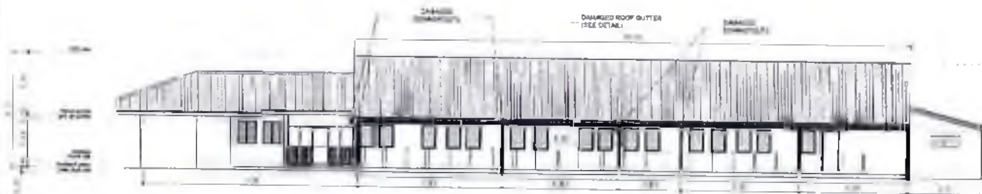
1 EXISTING CONDITION OF GUTTER & DOWNSPOUTS (REAR) SCALE 1:200 M
