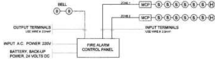
RISER DIAGRAM CONNECTION OF CONVENTIONAL FIRE ALARM SYSTEM (PICO AND BASEPORT TERMINAL BUILDING)
